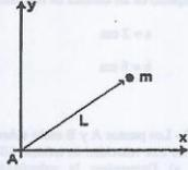
$$\tau_{\text{Neto}} = f_{\text{tangencial}}L = I_m \alpha_{\text{Angular}} = mL^2 \alpha_{\text{Angular}} \Rightarrow \alpha = \frac{f_{\text{tangencial}}}{mL} = 10 \text{ s}^{-2}$$
