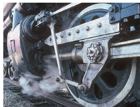
Figure 15.12 (Left) The pistons of an automobile engine move in periodic motion along a single dimension as shown in this cutaway view of two of these pistons. This motion is converted to circular motion of the crankshaft, at the lower right, and ultimately of the wheels of the automobile. (Right) The back-and-forth motion of pistons (in the curved housing at the left) in an old-fashioned locomotive is converted to circular motion of the wheels.
