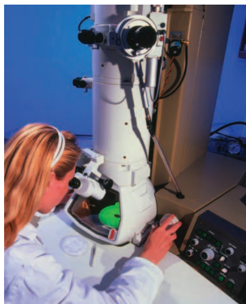
Figure 40.16 (a) Diagram of a transmission electron microscope for viewing a thinly sectioned sample. The “lenses” that control the electron beam are magnetic deflection coils. (b) An electron microscope.
