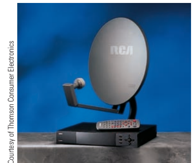
A satellite-dish antenna is a concave reflector for television signals from a satellite in orbit around the Earth. Because the satellite is so far away, the signals are carried by microwaves that are parallel when they arrive at the dish. These waves reflect from the dish and are focused on the receiver.
