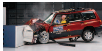
Figure 9.4 (Example 9.3) (a) This car's momentum changes as a result of its collision with the wall. (b) In a crash test, much of the car's initial kinetic energy is transformed into energy associated with the damage to the car.
