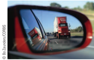
Figure 36.15 (Example 36.4) An approaching truck is seen in a convex mirror on the right side of an automobile. Because the image is reduced in size, the truck appears to be farther away than it actually is. Notice also that the image of the truck is in focus, but the frame of the mirror is not, which demonstrates that the image is not at the same location as the mirror surface.
