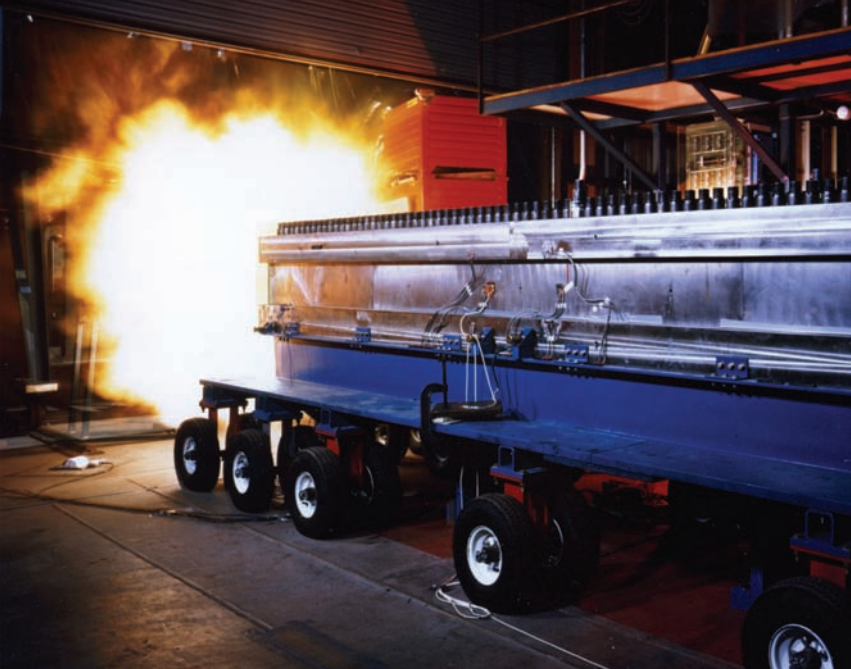
A proposed method for launching future payloads into space is the use of rail guns , in which projectiles are accelerated by means of magnetic forces. This photo shows the firing of a projectile at a speed of over 3 km/s from an experimental rail gun at Sandia National Research Laboratories, Albuquerque, New Mexico. (Defense Threat Reduction Agency [DTRA])
