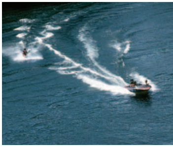
Figure 17.11 The V-shaped bow wave of a boat is formed because the boat speed is greater than the speed of the water waves it generates. A bow wave is analogous to a shock wave formed by an airplane traveling faster than sound.
